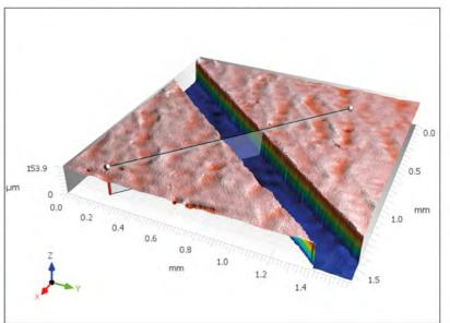
**INTERIOR** scratch measurement of an H175 windshield from the **OUTSIDE**!
